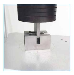
The double shear fixture is designed so the lower portion is supported by the machine table as a controlled, compressive load is put on the fastener. When the force is applied, a shear force at two fastener points is created. Complete procedure and apparatus for testing is specified in NASM1312-13.
